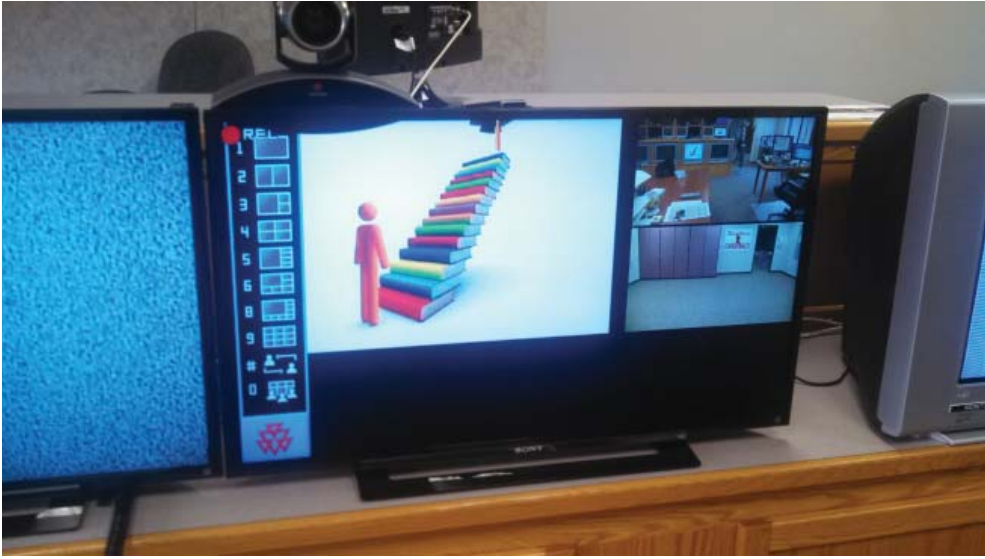
Option 6 is shown at left. This is considered a 1 by 5 layout with the 1 being the bigger box and 5 remote sites available on the side and bottom.
