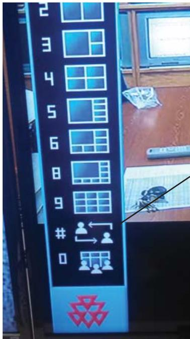
Close up of the screen option bar. Notice the # symbol. Pressing the # button allows you to move a remote site to a larger square (or full screen if in the full screen mode)
